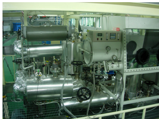
Fig. 2. The photograph of lead-bismuth corrosion test loop at KAERI (KPAL-I)
