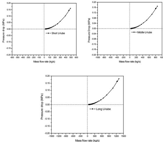
Figure 4. Pressure drop Vs mass flow rate during the transient.
