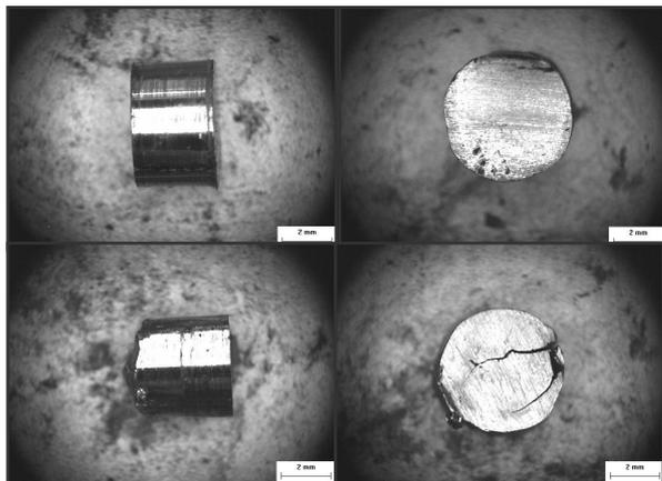
Figure 4. Observation results after decladding the cladding material of irradiated metallic uranium nuclear fuel.
