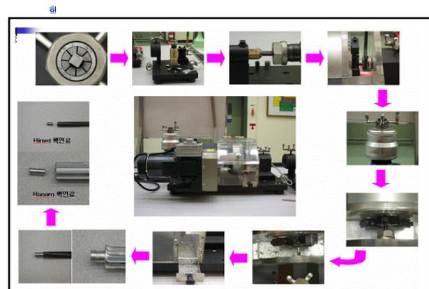
Figure 2. Decladding procedure for irradiated nuclear fuel.
