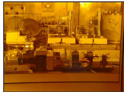
Figure 1. The appearance of a decladding machine for irradiated nuclear fuel.
