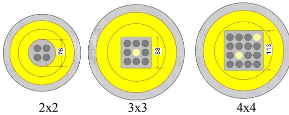
Figure 1. Layouts of the Flow Channels in CHTH
