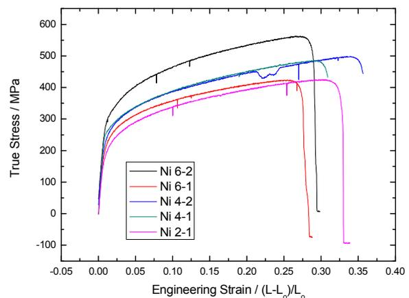
Fig. 3. Stress-strain curves for pure Ni electrodeposit as a function of the electrodeposit position in the length direction.
