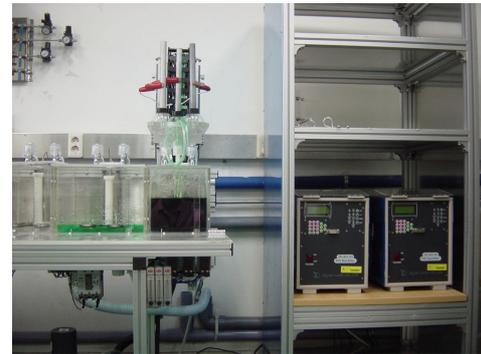
Fig. 2. Multiple electrodeposition system.
