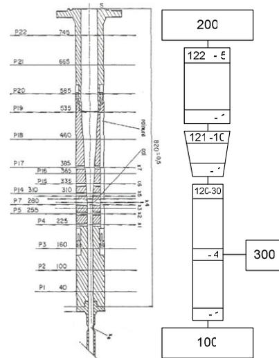
Figure 1. Moby Dick test section & noding diagram
