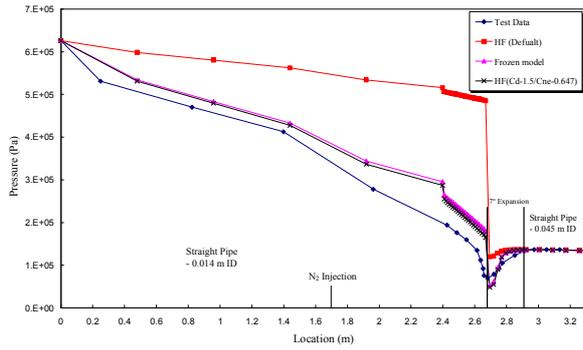
Figure 2. Comparison between pressure measurements and predictions for Moby Dick Test 3052
