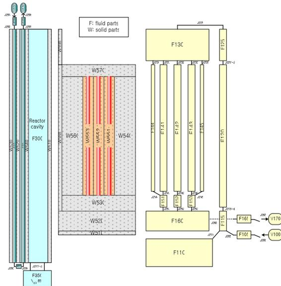
Fig.1 Fluid and Solid Parts Model of PMR 200MWth for GAMMA Code
