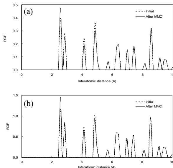
Figure 2. Cr-Cr radial distribution functions obtained from the MMC simulations of (a) Fe-5Cr and (b) Fe-15Cr alloy.
