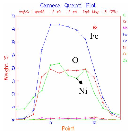
Figure 2 Quantitative analysis on CRUD layer
