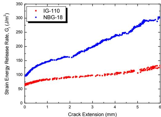
Figure 1. Strain energy release rate,  $G_I$ , curves as a function of crack extension for prestress-free IG-110 and NBG-18.
