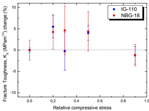
Figure 2. Relationship between fracture toughness and compressive prestress for IG-110 and NBG-18.
