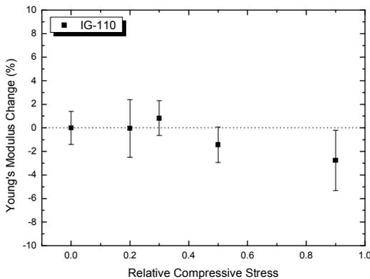
Figure 3. Relationship between Young's modulus and compressive prestress for IG-110 perpendicular to prestress axis.
