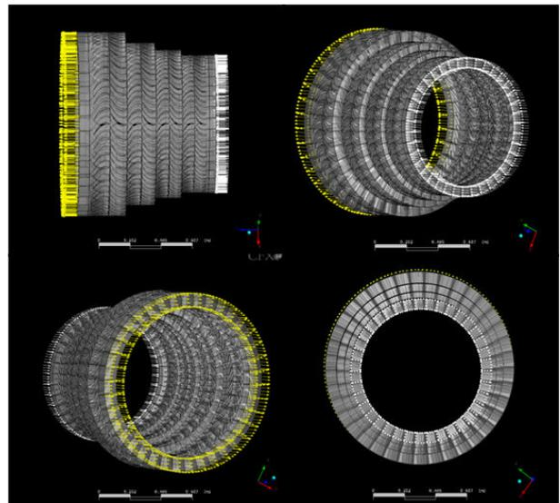
Figure 2. Three-dimensional SCO<sub>2</sub> turbine design with ANSYS BladeGen<sup>™</sup>.
