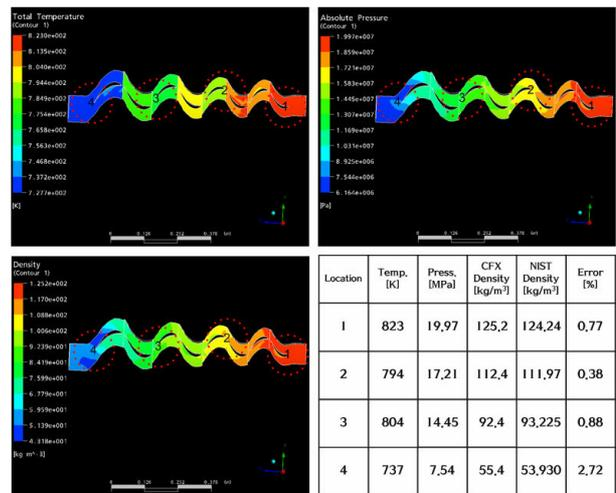
Figure 1. Comparison of calculated densities in CFX<sup>®</sup> and NIST.
