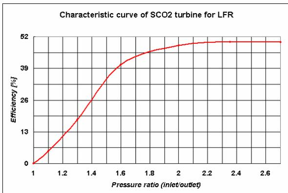
Figure 4. Efficiency variation with pressure ratio between inlet and outlet.
