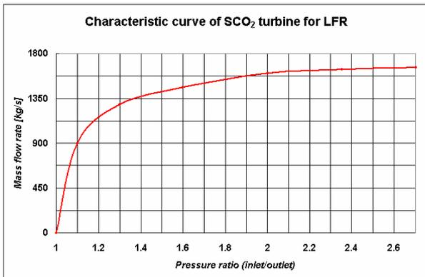
Figure 3. Mass flow rate variation with pressure ratio between inlet and outlet.
