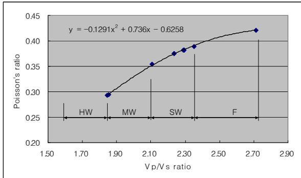
Fig. 2. Poisson's ratio as a function of Vp/Vs ratio
