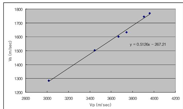
Fig. 1. Correlation of the elastic wave velocity of moderately and slightly weathered rock
