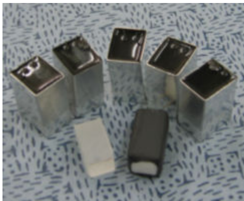
Figure1. Photos of the fabricated CsI/PIN structure detector.
