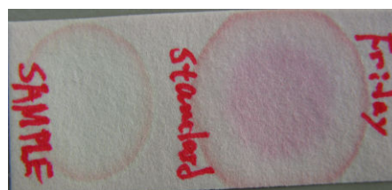
Figure 2. Results of Alumina Content Test: Alumina Standard Contains 10 ppm (Dark Color)
