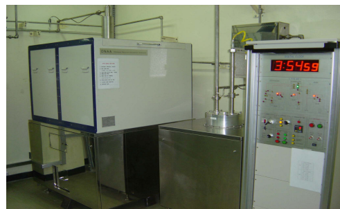
Figure 2. Picture of newly installed DNAA Counting System ; Shows (1)DNAA Counting System on left, (2)Sample loading station on middle, and PTS on right.
