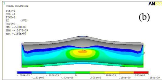
Figure 3. Thermal stress contours at the end of a) heating and b) cooling cycle
