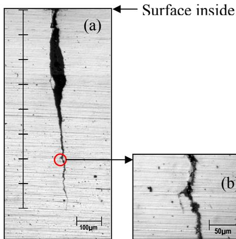
Figure 4 Cross-sections of thermal fatigue crack
