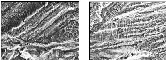
Figure 5. Fracture surface of thermal fatigue crack
