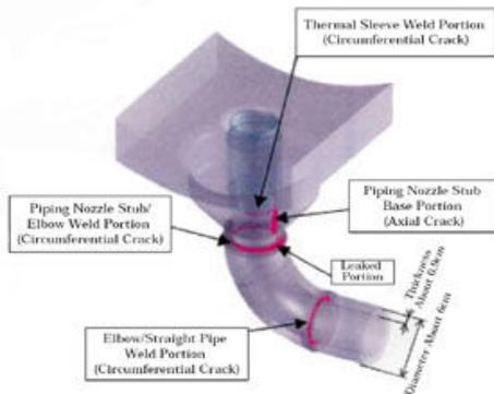
Figure 1. Outlet pipe of shell side of regenerative heat exchanger
