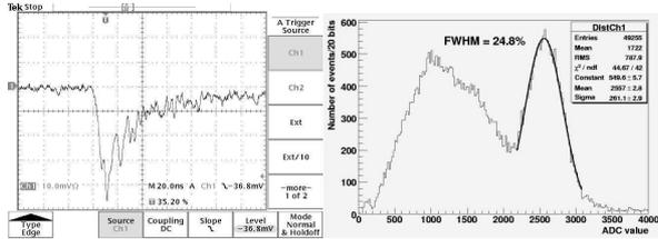
Figure 2. Raw pulse from the SSPM-LYSO coupling (a), and ADC distribution (b) for non-magnetic condition.
