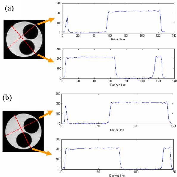
Figure 4. MRI Phantom image without (a) and with (b) the SSPM-LYSO coupling and the electronics in T2 weighted sequence.
