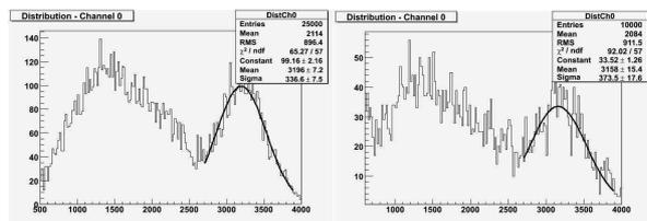
Figure 3. ADC distribution under the 3-T magnetic field (a), during the gradient echo MRI sequence (b).
