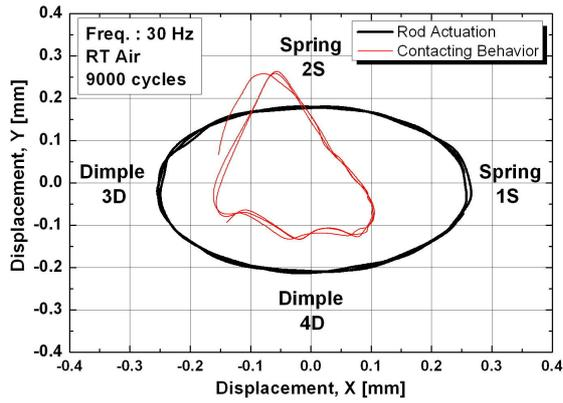
Figure 2. Variation of the contacting behavior of the fuel rod with an elliptical rod actuation in a 1x1 unit cell.
