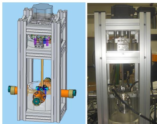
Figure 1. Schematic diagrams of the developed fretting wear test rig.
