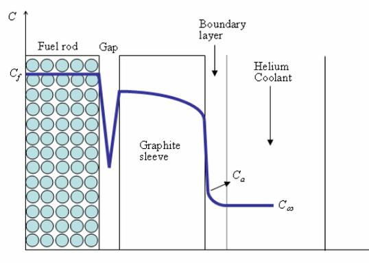
Fig. 1 Transport profile of fission products in a fuel element
