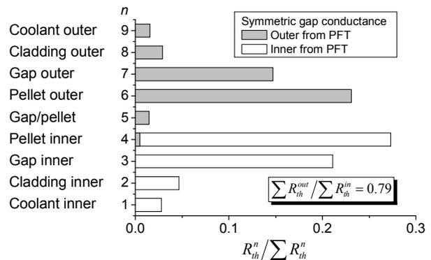
Figure 1 Thermal resistance at each component of KAERI-AF1 based on the peak fuel temperature (PFT).
