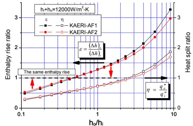
Figure 2 Enthalpy rise rate and heat split of outer channel to inner channel for KAERI-AF 12x12 fuel assembly with thermal barrier gap or not.
