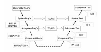
TG/OG: Test/Operation GuidelinePAT: Power Ascension TestHFT: Hot Functional TestCHT: Cold Hydrostatic TestRV: Reactor Vessel
