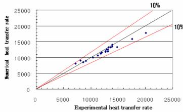
Fig. 4 Comparisons of heat transfer rate
