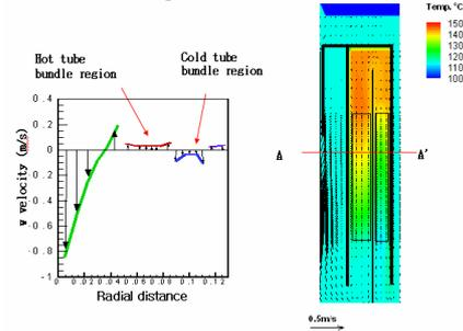
Fig. 5 Temperature and velocity field in the shell
