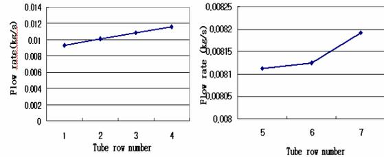
Fig. 6 Distribution of mass flow rate for each tube
