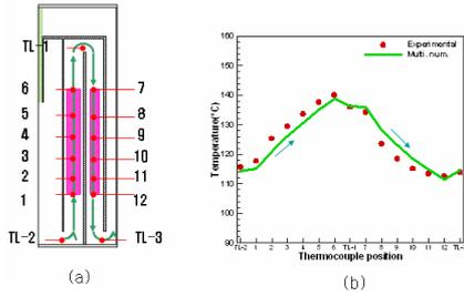
Fig. 3 Temperature distribution in the shell
