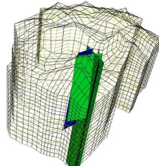
Figure 2. Grid structure and the fracture's location
