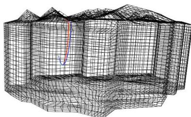
Figure 3. The groundwater pathway at the repository position
