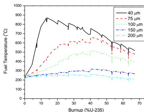
Figure 2. Fuel temperature histories with varying U-Mo fuel particle size.
