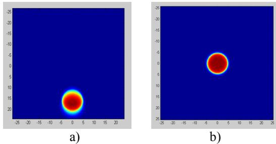
Figure 3. 2D images of uncorrected and corrected beams: MC simulation, magnified image by twice a) focused and uncorrected beam b) focused and corrected beam
