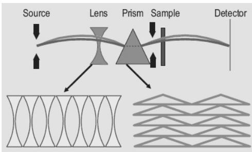
Figure 1. Cold neutrons collimation by multiple biconcave lenses and anti-gravity prism
