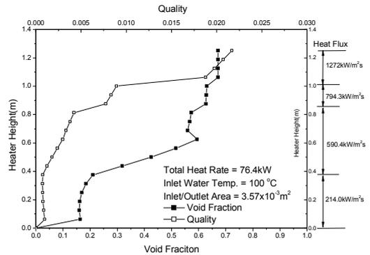
Figure 3. Calculated void fraction and quality.
