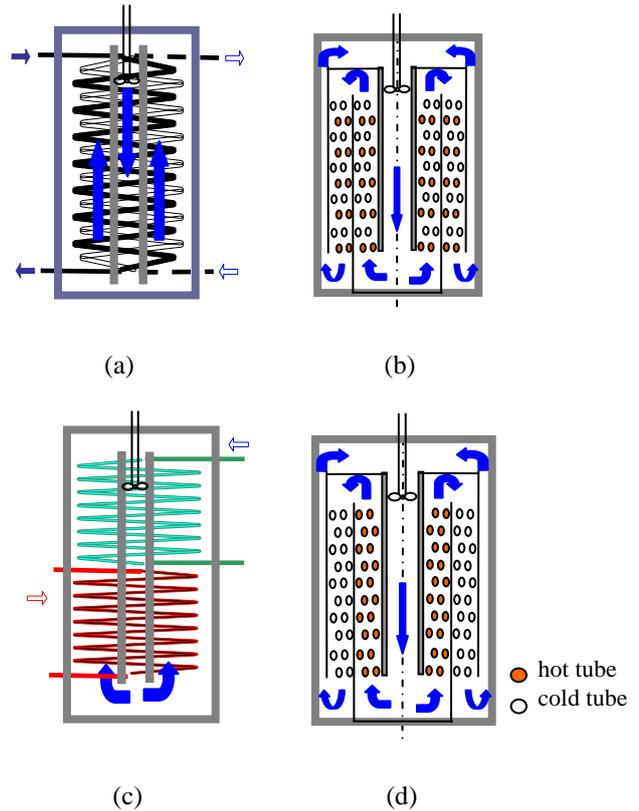
Figure 1. Tube bundle configuration of the DTBSG
