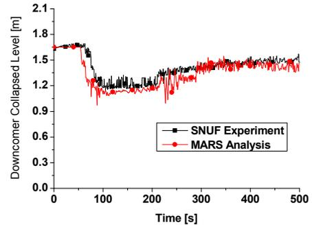
Figure 3. Downcomer Collapsed Water Level
