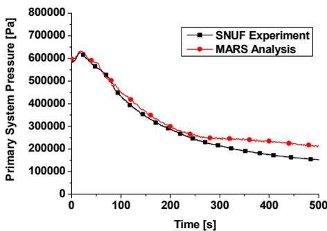
Figure 2. Primary System Pressure
