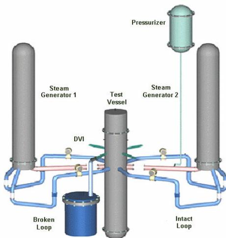
Figure 1. Schematic of the SNUF facility.
