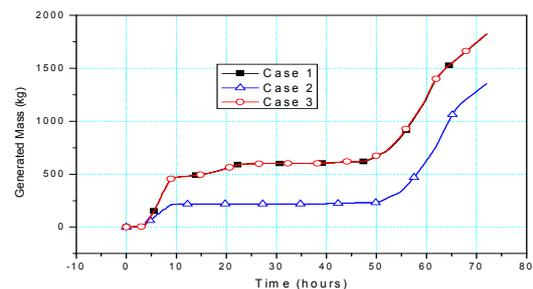
Figure 1. Total Amount of Hydrogen Generated in the Calandria Vessel and Calandria Vault
