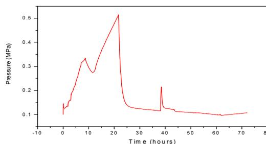
Figure 4. Pressure in Upper Dome for the Case 3-A
