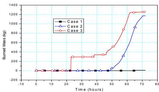
Figure 2. Total Amount of Hydrogen Burned in R/B
