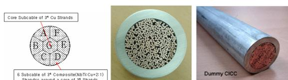
Figure 4. Superconducting cable-in-conduit conductor (CICC) for bus-lines.
