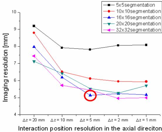
Fig. 2. Imaging resolution of the Compton camera for different segmentations of the absorber
