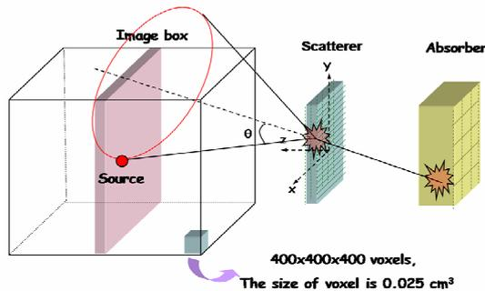
Fig. 1. Diagram of the Compton camera with a back-projected cone for image reconstruction
