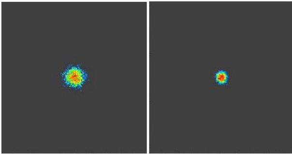
Fig. 3. Compton camera images for the case of current system (left) and the improved system (right)
