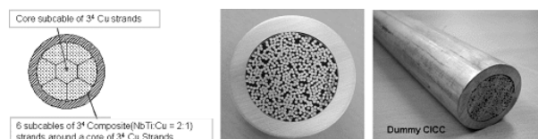
Figure 4. Superconducting CICC for bus-line
