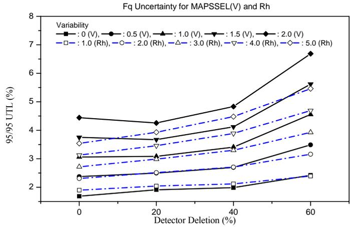
Figure 2. Peaking Factor Uncertainty vs. Fraction of Inoperable detectors for 5 element Rh and MAPSSEL 6 Va detectors
