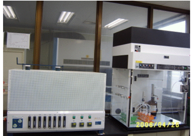
Fig. 2. The combustion furnace with auxiliaries for measuring the radioactivity
