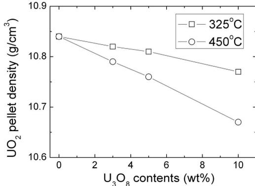
Fig. 2. The  $UO_2$  pellet density changes according to the  $U_3O_8$  powders contents.
