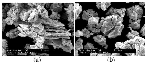
Fig. 1. The SEM images for  $\text{U}_3\text{O}_8$  powders which are obtained by oxidizing the  $\text{UO}_2$  pellets at (a) 325°C and (b) 450°C.
