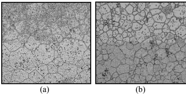
Fig. 3. The grain morphologies of 5wt% of  $U_3O_8$  containing Al-doped  $UO_2$  pellets. (a) 325°C (b) 450°C
