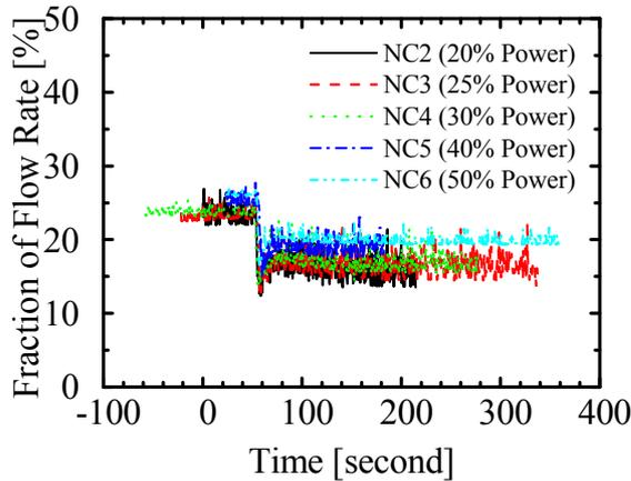
Fig. 1 Core Flow Rates for the Natural Circulation Tests
