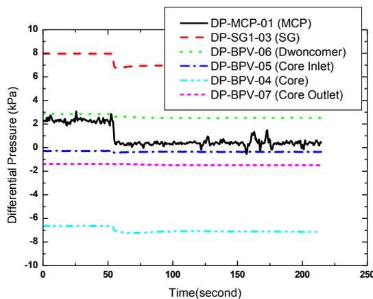
Fig. 2 Differential Pressure Distribution in the Primary Loop for the Test of NC2
