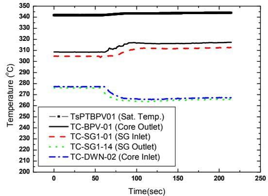
Fig. 3 Fluid Temperature Distribution in the Primary Loop for the Test of NC2
