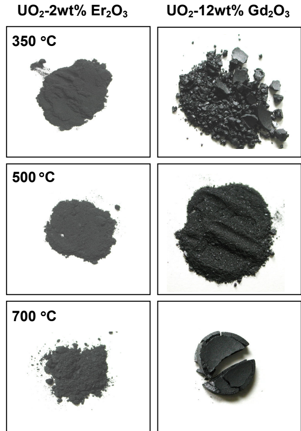
Fig. 3. Morphologies of the \text{M}_3\text{O}_8 powder obtained by oxidation of sintered \text{UO}_2\text{-2wt\%Er}_2\text{O}_3 and \text{UO}_2\text{-12wt\%Gd}_2\text{O}_3 pellets at various temperatures.
