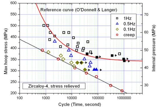
Fig. 2 Stress-life diagram of zirconium cladding with the loading frequency.
