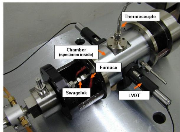
Fig. 1 The cyclic pressurization device for testing low cycle fatigue
