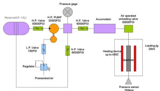
Fig. 1 Schematic illustration of rapid pressurization device for simulating RIA
