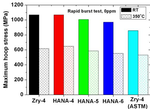
Fig. 3 Maximum burst hoop stress of the as-received HANA cladding under the rapid pressurization test.
