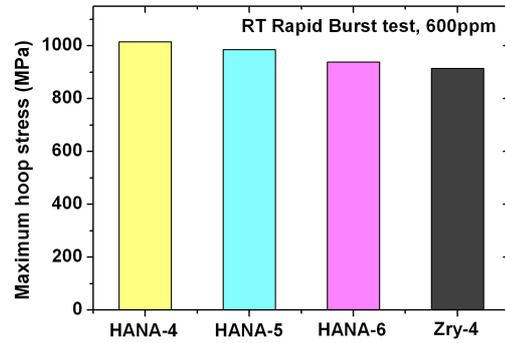
Fig. 5 Maximum burst hoop stress of the hydrided HANA cladding under the rapid pressurization test.
