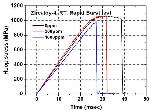
Fig. 4 Time-pressure profile of Zircaloy-4 cladding with the hydrogen content.
