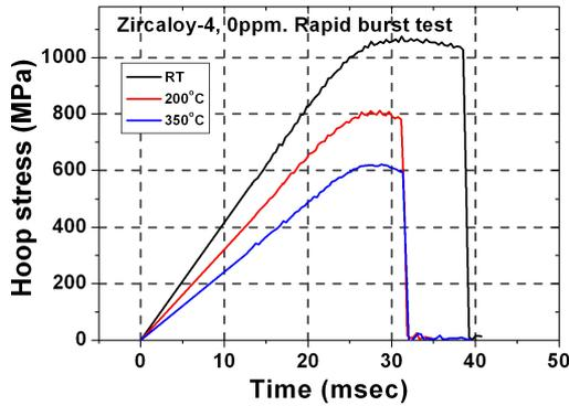
Fig. 2 Time-pressure profile of Zircaloy-4 cladding with the test temperature.
