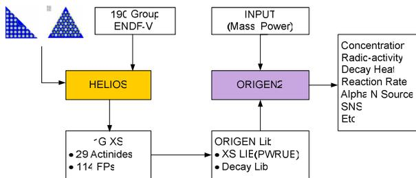
Fig. 1. Decay Heat Calculation Procedure with HELIOS/ORIGEN.
