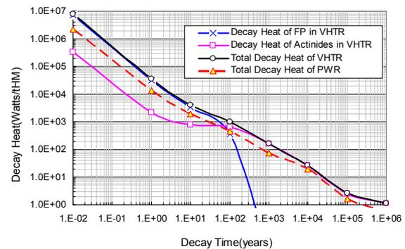
Fig. 4. Decay heat vs. cooling time.
