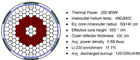
Fig. 2. PMR200 Core Design & Parameters.
