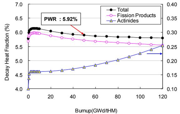
Fig. 3. Decay heat fraction vs. burnup.
