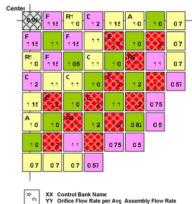
Fig. 2. Loading pattern of a Equilibrium Core with Control Banks and Orifice Flow Rates
