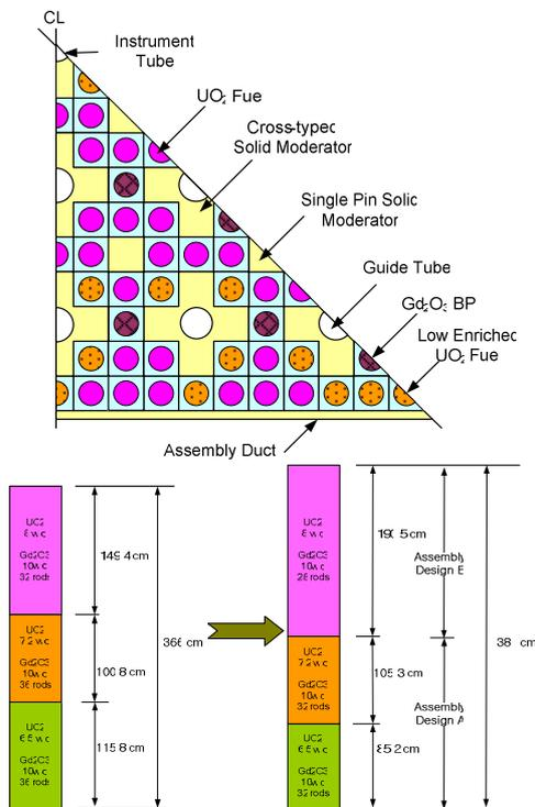
Fig. 1. Cross-sectional view of assembly model and axial zoning of fuel and burnable poison rod.
