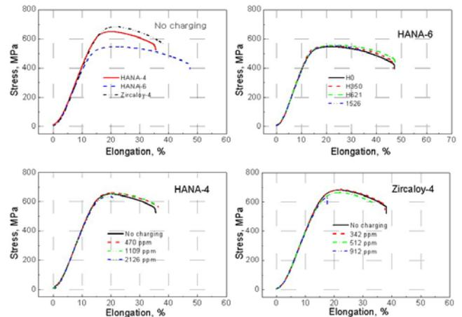
Fig.1. Stress-elongation curves of the claddings at room temperature
