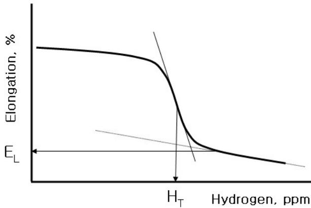
Fig.2 Diagram for the explanation of ductile-brittle transition of the cladding with hydrogen content
