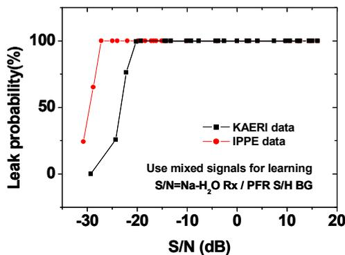
Figure 4. Leak probability tested by the developed acoustic leak detection tool.
