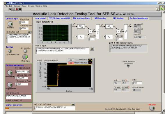
Figure 2. LabVIEW panel of the acoustic leak detection system developed in KAERI.
