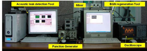
Figure 1. The On-line acoustic leak detection system developed in KAERI.
