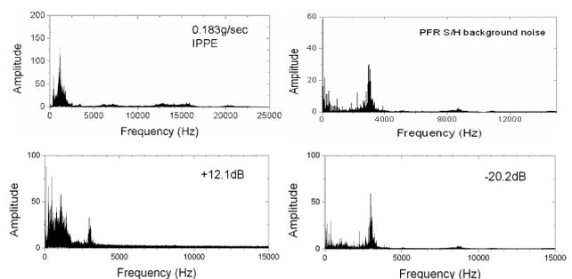
Figure 3. Typical FFT analysis results of the SWR acoustic noises mixed with PFR S/H background noise obtained by the KAERI SWR experiments for water into a sodium leak and by the IPPE.
