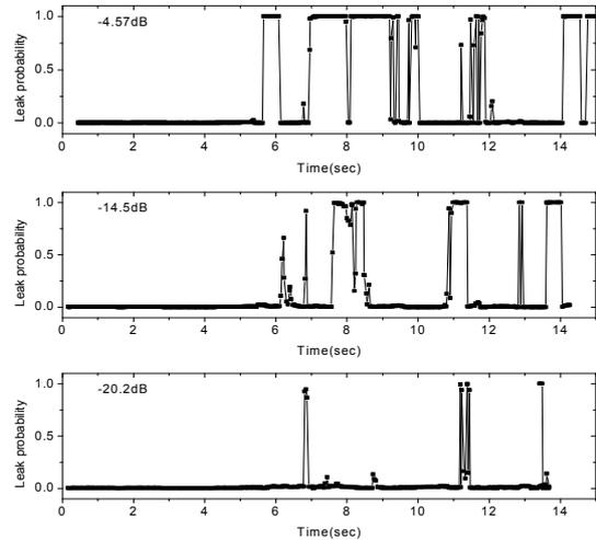
Figure 5. Leak probability tested by the developed on-line acoustic leak detection tool.
