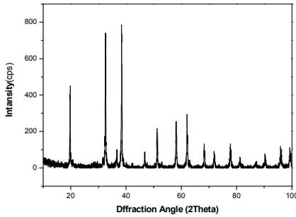
Fig.2.A typical X-ray diffraction result for the  $UAl_2$  specimen formed by an annealing. The measured relative densities of the annealed specimens are shown in Table.1.
