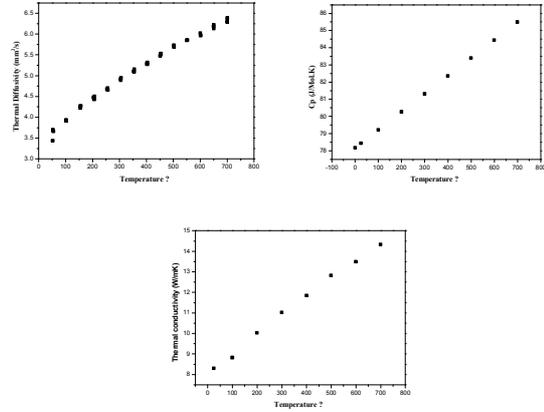
Fig.3. Thermal conductivities, specific heat measured and Thermal diffusivity measured for the  $UAl_2$  specimen formed by an annealing at 1200 °C for 10 hours with zircaloy mould.
