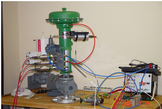
Figure 2 AOV Test Facility
