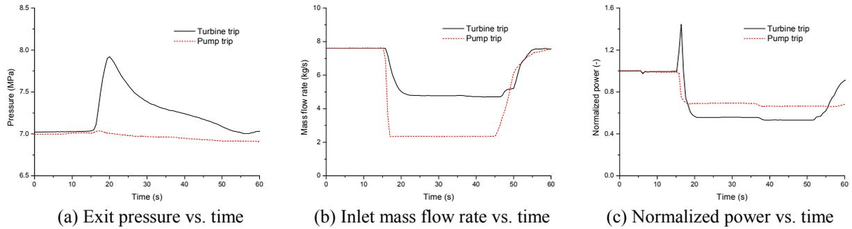
Figure 3. Boundary conditions for the turbine trip and the pump trip.
