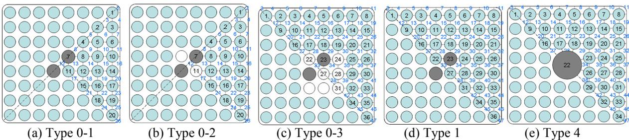
Figure 1. The fuel assembly type and its MARS input model: Channel and rod numbers are given.
