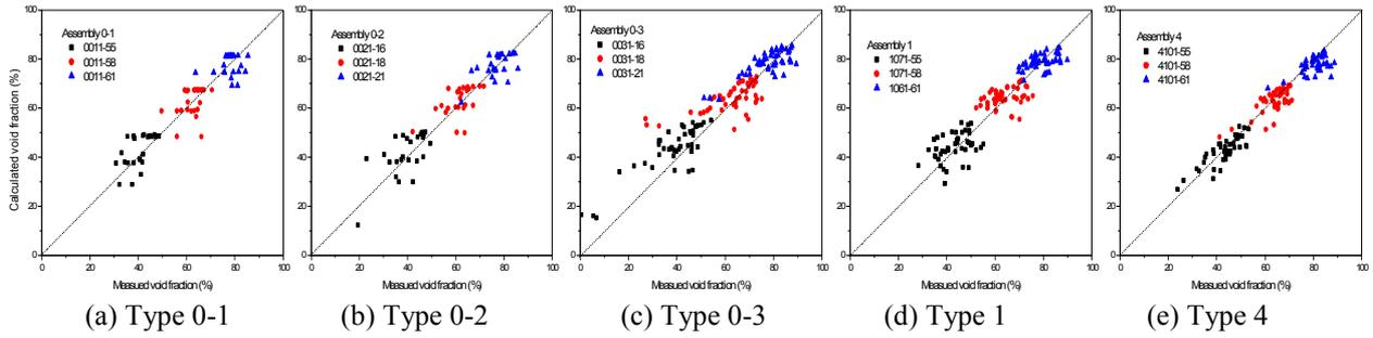
Figure 2. Comparison of the steady-state void fractions at the subchannels above the channel exit.
