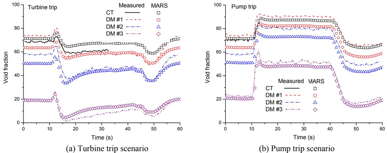
Figure 4. Comparison of the transient void fractions: Turbine and pump trip cases
