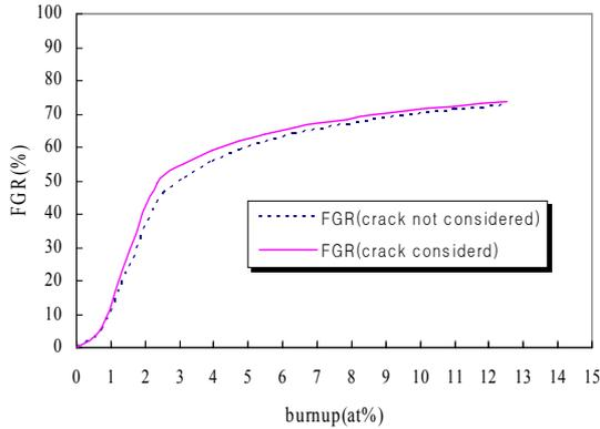
Figure 2. Fission gas release rate according to the crack
