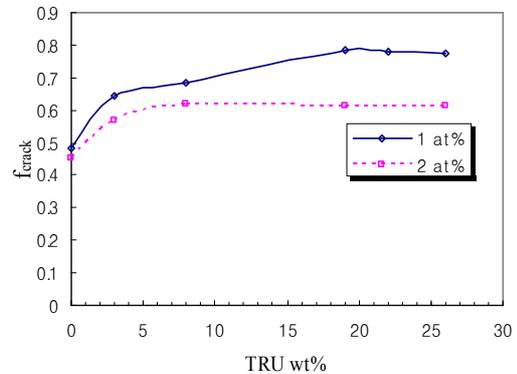
Figure 1. Anisotropy factor,  $f_{crack}$ , as a function of TRU wt% according to a burnup
