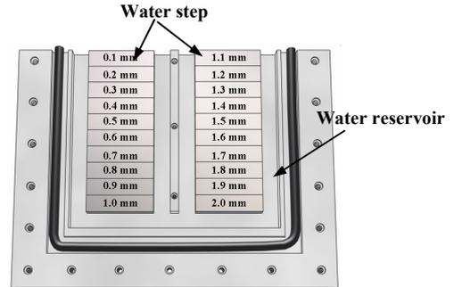
Figure 1. Schematic Diagram of Al Block
