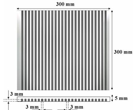
Figure 2. Schematic Diagram of Grid
