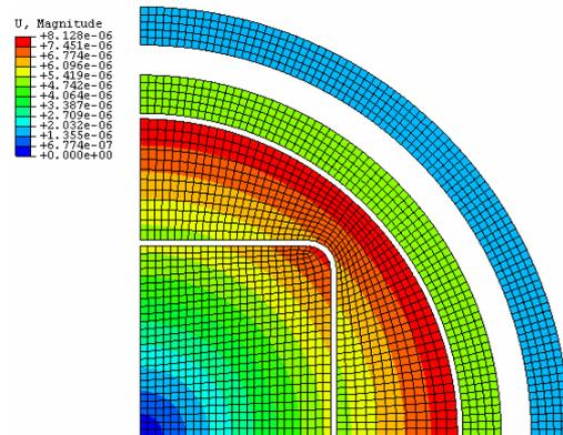
Figure 6. Displacement Contour of the Capsule
