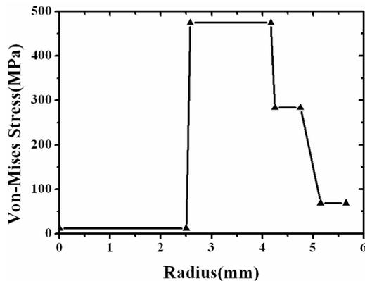
Figure 5. Stress Profile of the Capsule in the Radial Direction
