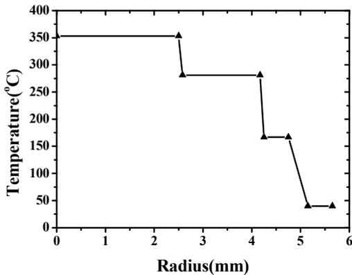
Figure 4. Temperature Profile of the Capsule in the Radial Direction
