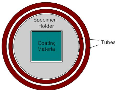
Figure 1. Cross-sectional View of the Irradiation Capsule
