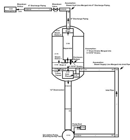
Figure 2. RELAP5 nodalization for CE-KDL test
