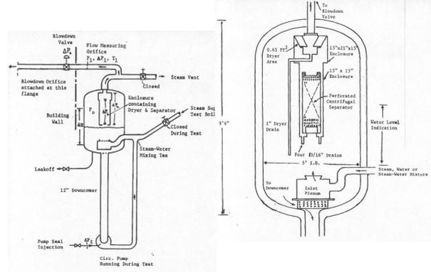
Figure 1. MSLB test loop and vessel of CE-KDL
